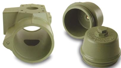
The XL Commando range solves aggressive corrosion problems. It works where stainless doesn't. A proprietary heat treatment with CG941 fluoropolymer impregnates the body making it impervious to corrosion. The steel pinion is also fluoropolymer coated. Field service has shown that the Commando actuators outperform other actuators in corrosive environments.
